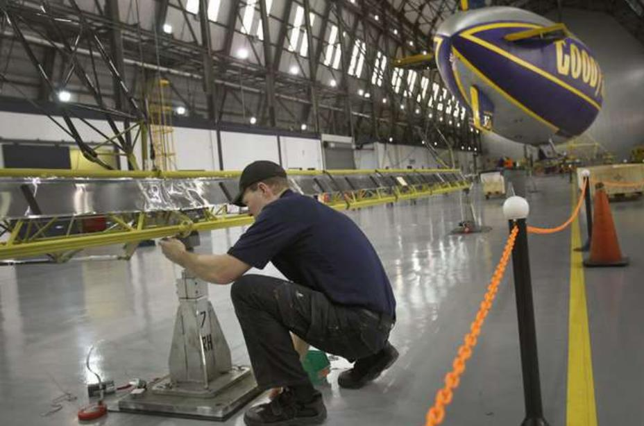
Structural mechanic Markus Draeger fastens a longerone to the triangle section as part of the interior structure of the new craft
