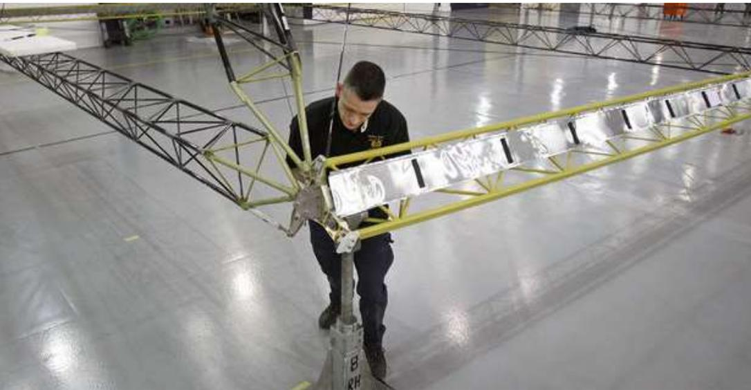
Airship mechanic Tom Bradley attaches a tensioning cable to a triangle section as part of the interior structure the airship
