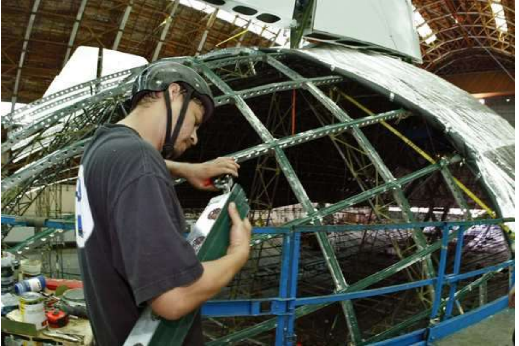
Fredy Zuniga trims a piece of the airship's aft section framework. "Because of the curves, every single piece has to be custom cut and fitted," Zuniga says.
