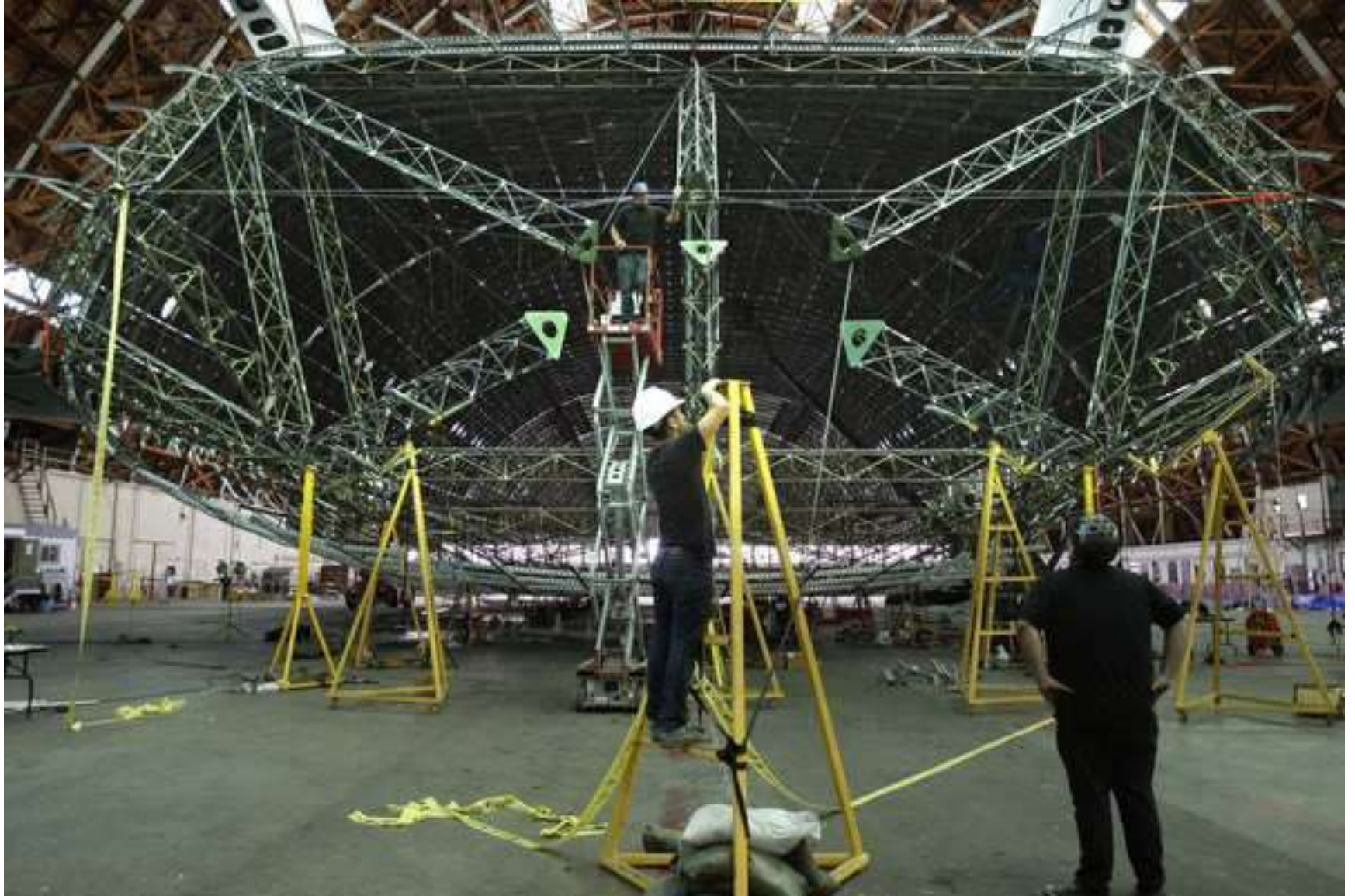
Craftsmen assemble the aft portion of Worldwide Aeros' blimp-like airship under construction in a World War II-era blimp hanger in Tustin.
