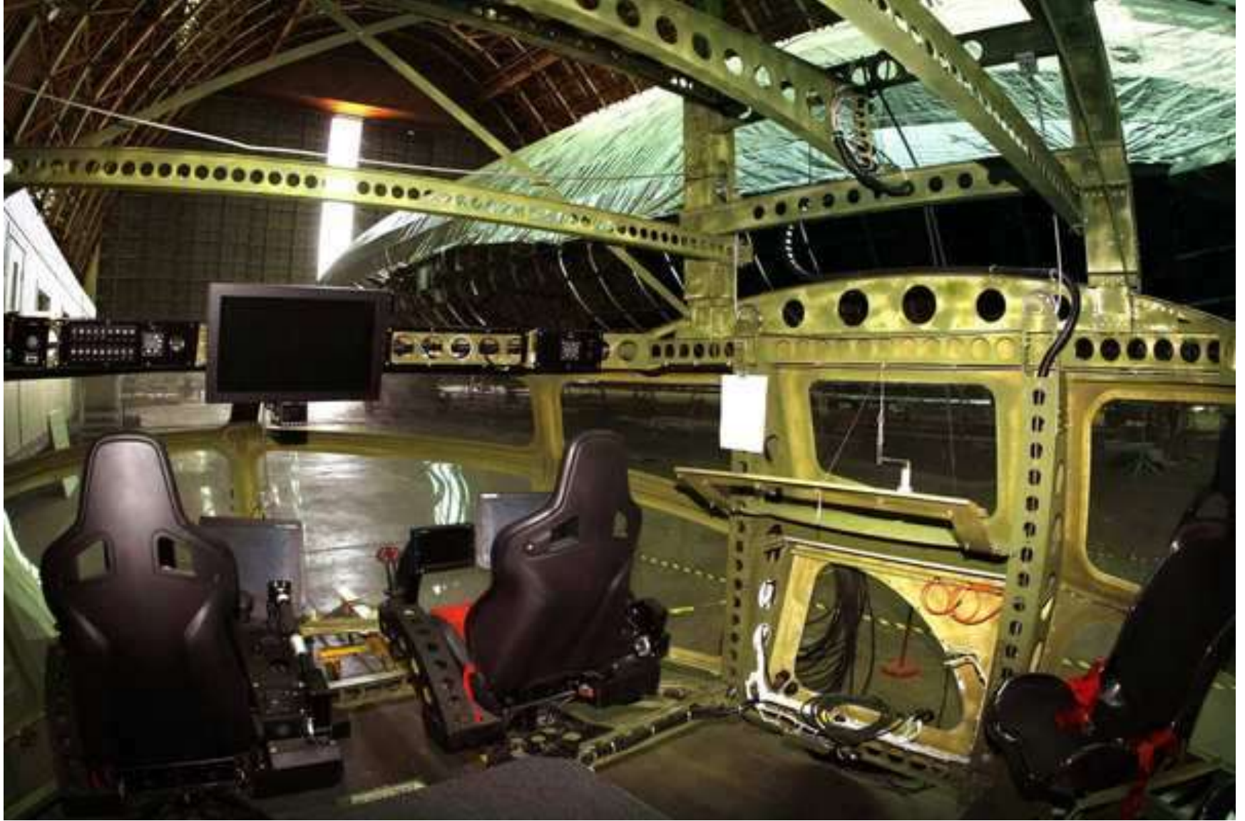
The cockpit sits on the floor next to the partially assembled airship. It will be installed beneath the craft.
