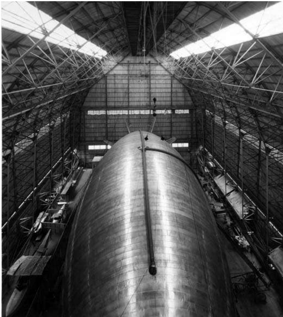
Looking toward rudder end of ship showing inflation tubes on top of ZMC-2 Charles Rosendahl LTA Collection – University of Texas - Dallas
