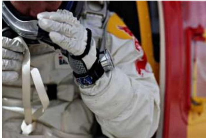
Once Baumgartner depressurizes the vessel and opens the door to step off, his full-pressure suit and helmet – what engineers call a “pilot protective assembly,” or PPA – will be his only life-support system until he reaches the safety of the lower atmosphere.
