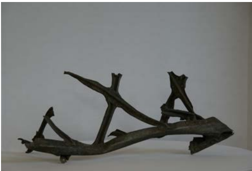
One of the USS Shenandoah girders recovered from the crash site. The image can be rotated 360°
