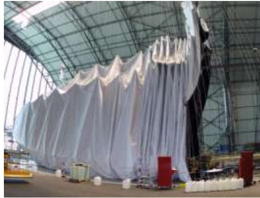
Slipping the Hull over the Frame
