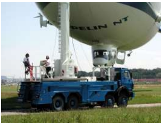
Zeppelin at Mobile Mooring Mast
