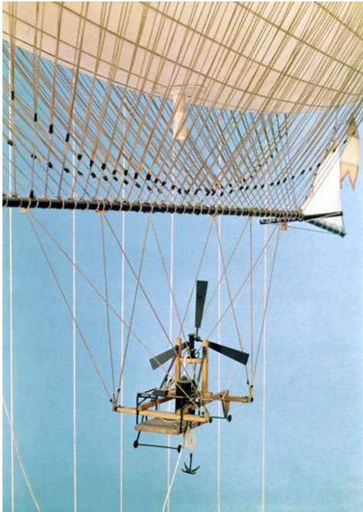
Detail of the car of the dirigible used in the first successful application of mechanical power to flight. The power unit was a single cylinder steam engine constructed by the French designer Henri Giffard.
